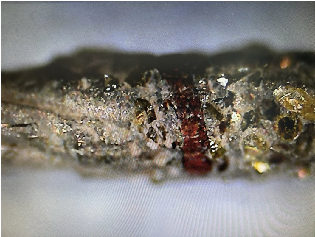
Fig. 6 — Optical micrograph of the fracture zone showing reddish-brown iron oxide deposits (indicated by arrow) within the damaged matrix, consistent with corrosion-assisted degradation of the steel core.
